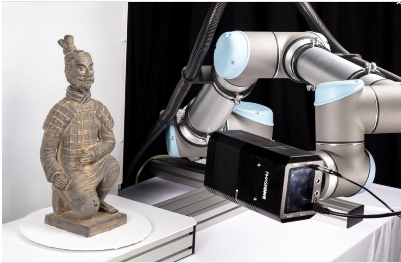
Figure 8. doi The CultArm 3D automated imaging system (© CultLab3D).
