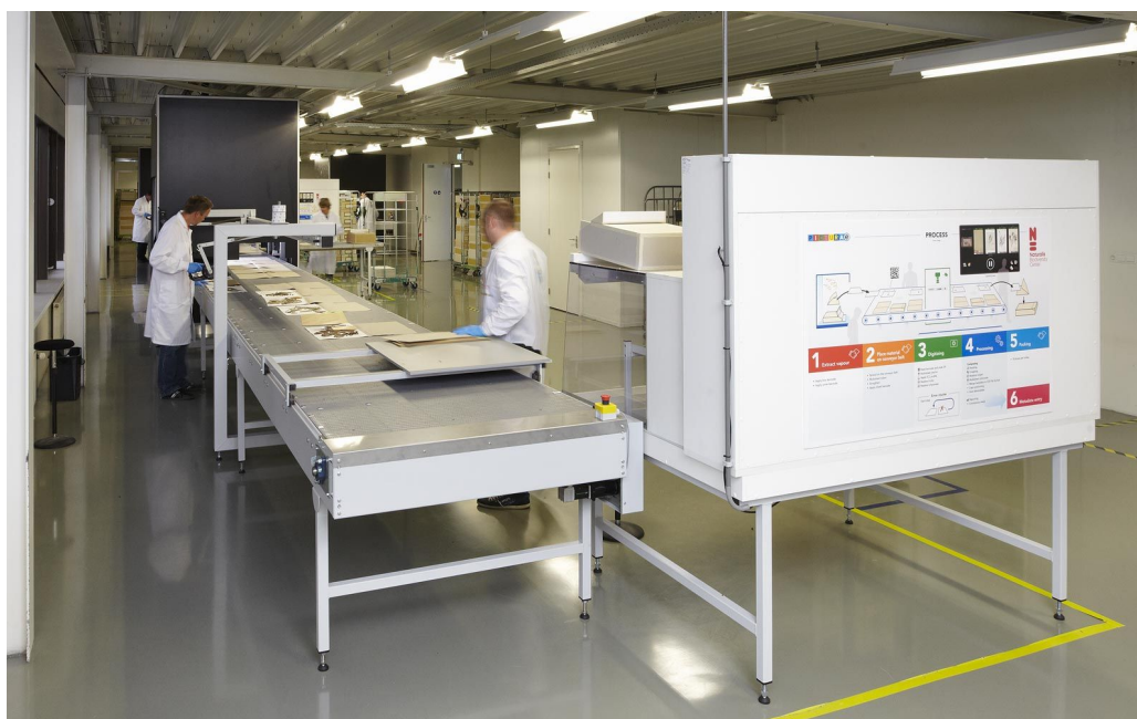
Picturae's conveyor belt set up for the project at Naturalis. The black structure contains the camera and lights, showing the distance of camera to subject. Greater distance can only be achieved in spaces that have high ceilings. (Image copyright Picturae)
