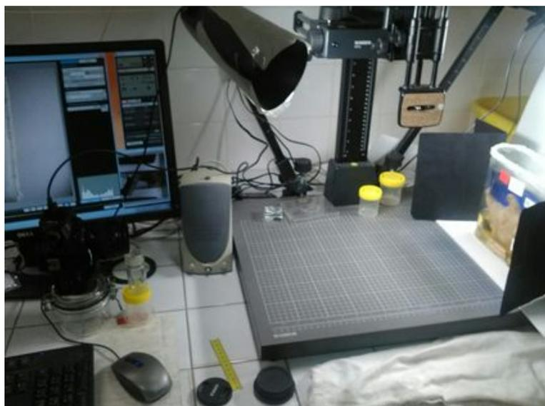
Imaging station for sealed containers: monitor with live view and camera left, specimen and background right. Black paper is used to limit lighting to relevant parts. (Image copyright MNHN)
