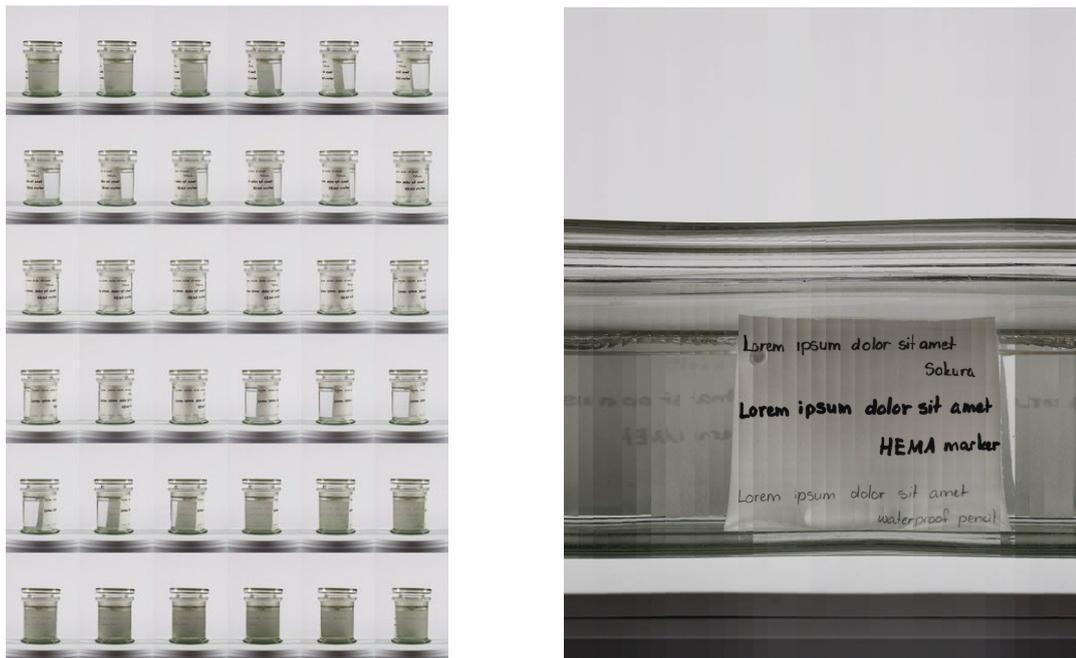
Output from test at Picturae with Nikon 800D camera. Left: the captured images. Right: the stitched crops of the center of each frame.
