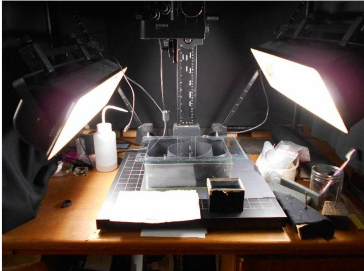
Photography setup for dry imaging of liquid preserved specimens: the specimen is placed on the glass pane, which is raised from the background, to ensure a blurred background. The camera is facing down on a copy stand and two lights are on either side. (Image copyright MNHN)
