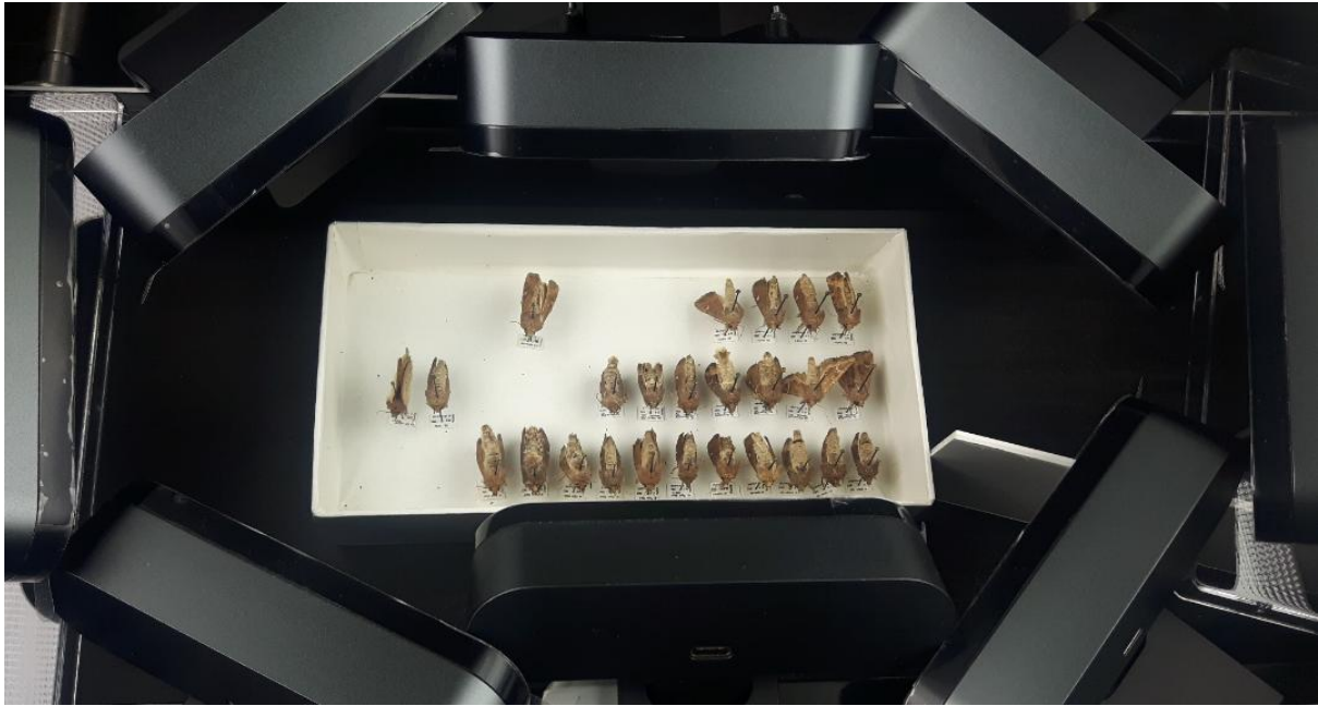
Figure 4. An example of the setup of the imaging area of the conveyor belt driven insect digitisation system with a single layer camera array of 8 webcams for unit tray digitisation
