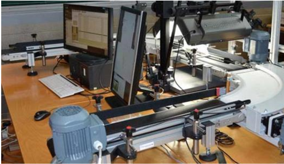
Figure 1. The conveyor belt driven pinned insect digitisation system (Tegelberg et al. 2014, 2017).
