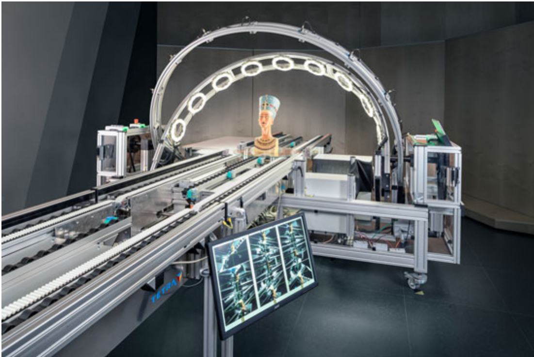
CultLab3D in action, showing the double arcs and conveyor belt. Source: https://www.cultlab3d.de/index.php/cultarc3d/
