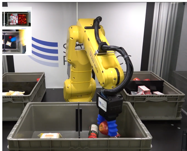
Soft Robotics gripper, still from video (00:41) just before release of object. Source: https://youtu.be/Pxd5-ZD9XcQ
